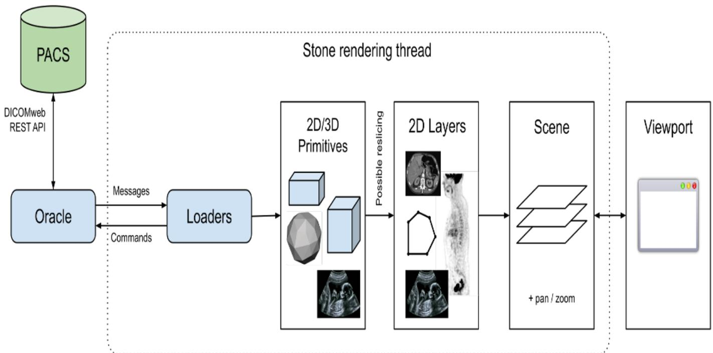
High-level view of the components of the PACS Imaging library. The Oracle abstracts the runtime environment. The Loaders are responsible for loading the graphical primitives that have to be displayed. These primitives are converted into a set of 2D Layers (in particular, primitives corresponding to 3D volumes can be sliced along a cutting plane). The Layers are then assembled as a Scene that is finally composed onto the rendering surface of the Viewport. The user can
